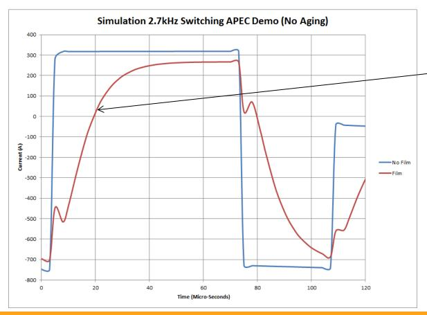
Adding 1.5mF with 2x Power Ring capacitors filters high frequency components from electrolytic current pulses
