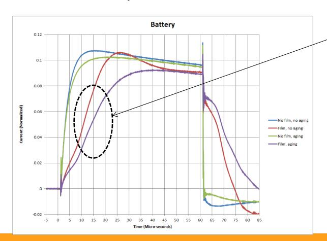
Adding film changes pulse structure much like simulation
