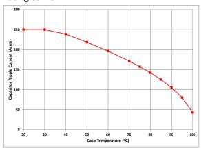
Ripple current versus case temperature for 10,000 hour life with continuous operation at 450V.
