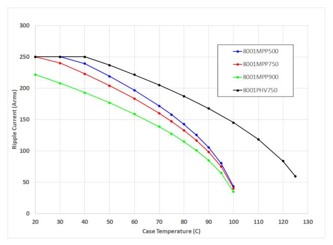
Ripple current versus case temperature for 10,000 hour life with a typical drive cycle and the average operating voltages listed below:
