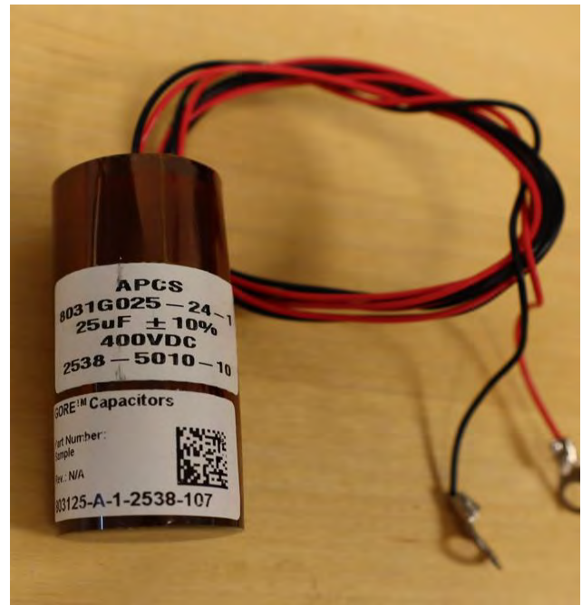
Fig. 2 Photograph of a PTFE-based film 400Vdc capacitor used for life testing.
